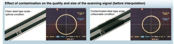
High insensitivity to contamination by use of a new scanning principle.
