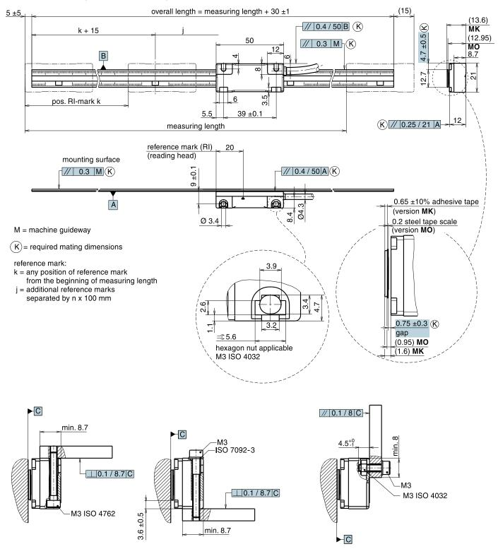
MS 40.xx MP steel tape scale in aluminum carrier with clamping element, carrier with adhesive tape
